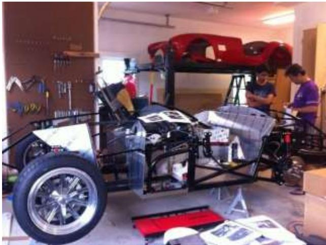
I assembled various subsystems: pedal box, fuel system, brake lines, suspension, steering, dashboard, upholstery, insulation, wiring harness, and more.
