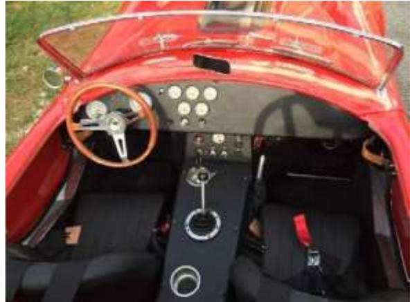
We made several custom mods including an under-dash console, cup holders, a signal stalk. I was responsible for designing, fabricating, and installing the center console.
